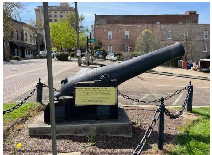
9" Naval gun designed by John A. Dahlgren in the early 1840's and cast at the Fort Pitt Foundry in 1862. It weighs 9,200 lbs. and took a crew of 16 to man it.
