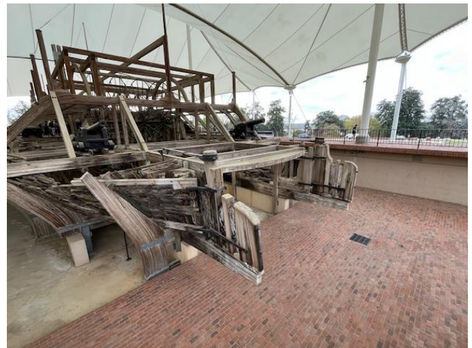
Rudders on either side of the paddle wheel were used to steer the gunboat. These wooden rudders were controlled by cables attached to the wheel in the pilothouse.
