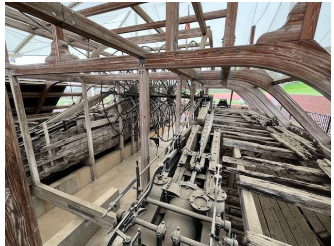
Piston, oscillating arm, and 15' wide by 22' diameter paddle wheel. The paddle wheel churned within a well near the back of the boat.
