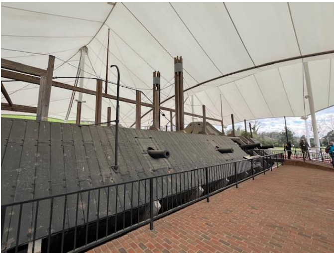
Iron cladding and cannon ports on starboard side.
