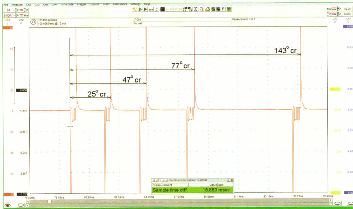
ATS scope pattern zoomed in on injection cycle during regeneration.
