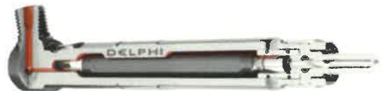
Delphi DF13 Direct Acting Diesel Injector (Product Cut-away)
