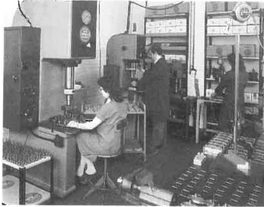
Assembly is checked at every stage of the production process in a room equipped with the appropriate presses and mounting equipment.
