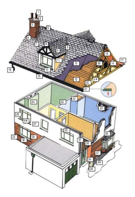
Ridge ventilation 5 Ridge board Slates/tiles 8 Valley guttering 9 Dormer projection Dormer flashing 10 Dormer cheeks 11 12 Sarking Roof felt 13 Trusses 14 15 Collar 16 Insulation 17 Parapet gutter Eaves guttering 18 Rainwater downpipe 19 20 Verge boards / skews 21 Soffit boards 22 Partition wall Lath / plaster 23
