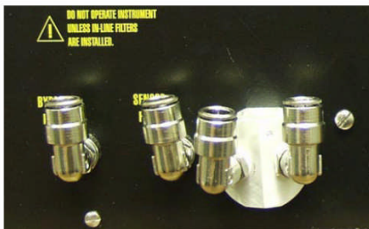
Back Panel of Control Unit, Showing Flow Inputs on Left (Unchanged), and Revised Flow Exhaust on Right Using Parts from FDMS Kit.
