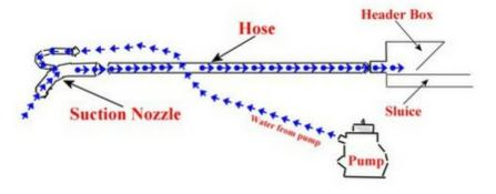
Suction dredges utilize a high-pressure gasoline powered water pump to suck up water, gravel and gold, and inject this material into a sluice through a header box. The header box dampens the rush of water and gravel so that it flows evenly into the sluice. The sluice then expels the worthless gravel and retains the gold. The sluice captures the gold behind the riffles.
