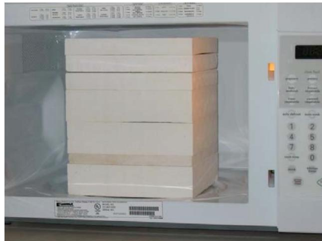
After 45 minutes, open the microwave door and, wearing heat proof gloves, safety glasses and apron, carefully lift the entire kiln out, holding it by the base. Hold the kiln with both hands
