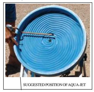
The aqua -jet is positioned simply by bending it to get the stream of water aimed into the
