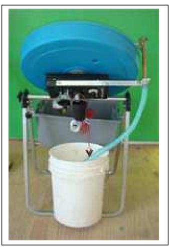
The spraybar mounts on the back of the drive unit on the two studs with wingnuts. Note that you should use care when hooking the spraybar and aqua-jet. in the wheel.
