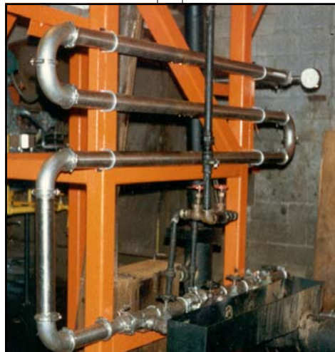
10,000 pound per hour capacity, Dual In Line Coagulators, complete with serpentine coil. Stainless steel construction is standard.
