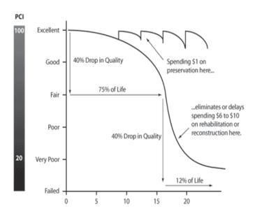
**Figure 1.** Pavement Deterioration/Rehabilitation Relationship
