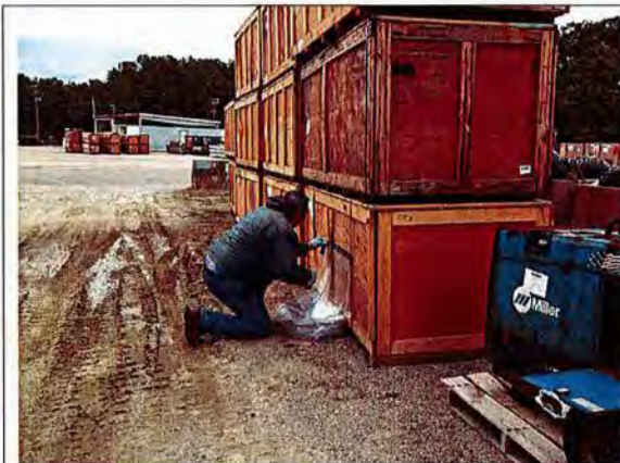
Washdown sampling for untreated wood.
