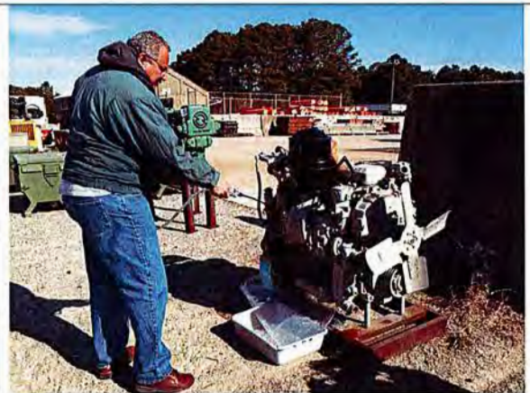
Washdown sampling for engine block.
