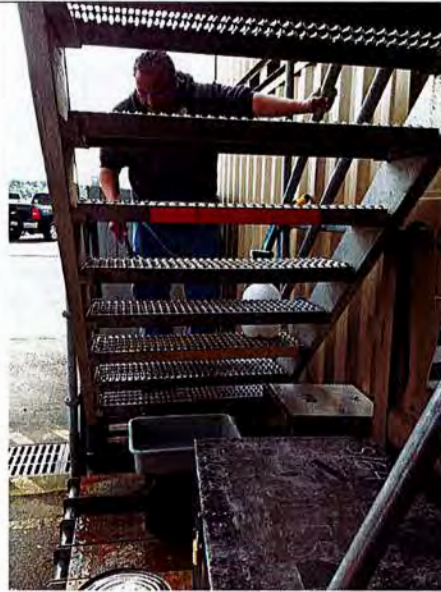
Washdown sampling of galvanized stair steps.
