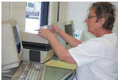
The results of each DPE Test are objectively evaluated using a reflectometer.
