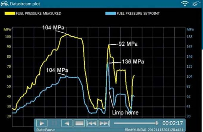
Launch GDS scantool recording of the actual rail pressure (yellow trace) vs desired pressure (blue trace). Please note the different MPa scales.
