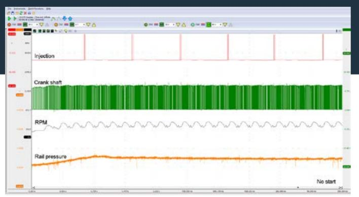
ATS 5004 3 channel recording with added RPM trace for TDC detection.
