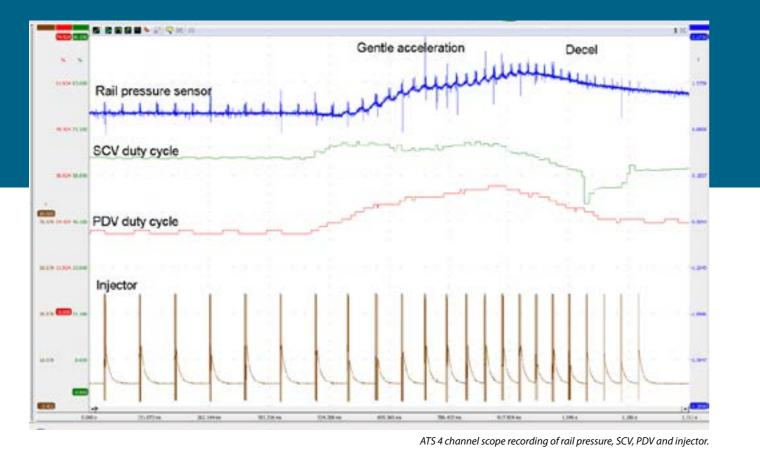
First we accelerated gently, just like the recording with the scantool. Both the SCV and the PDV traces do not move to ridiculous values, meaning that the ECU has the rail pressure under control, i.e. the actual rail pressure follows the desired rail pressure.
