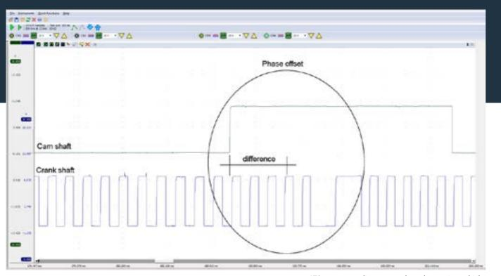
The next pattern is recorded on the running identical vehicle. Please note the phase offset between the cam and crank and compare with the not going vehicle.
