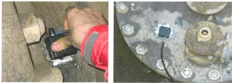
Figure 2: Example SMS Acoustic Sensor Glued to Flange
