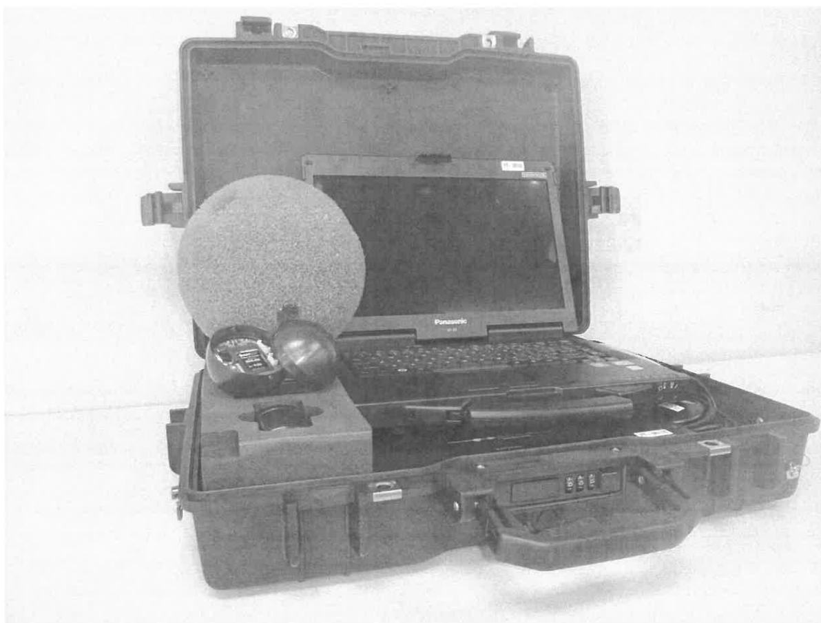
Figure B.1: SmartBall Core and Foam Shell a with SmartBall Receiver (SBR)
