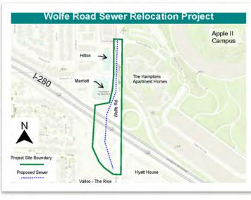
Cupertino Sanitary District is required to relocate its existing 15-inch sanitary sewer within the Caltrans right of way at Wolfe Road in Cupertino due to the planned I-280 interchange project.
