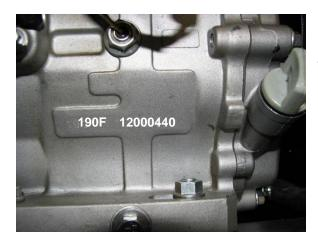
The engine serial number can be found stamped on the engine block near the oil dipstick. It is visible when the maintenance door is removed.
