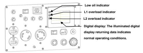
When connecting appliances, be aware of the electrical requirements of each appliance, and how much current will be available through each generator receptacle. For example, the L5-30R connector will conduct up to 30 amps. Connecting a combination of appliances that draw more than 30 amps total will overload the circuit. In that case you would connect those appliances to a combination of receptacles, based on the amperage required for each appliance.
