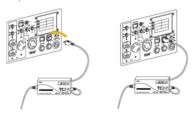
**6.** Charge the battery for 3 hours or until it is fully charged. After the battery is fully charged, disconnect the battery charger.
