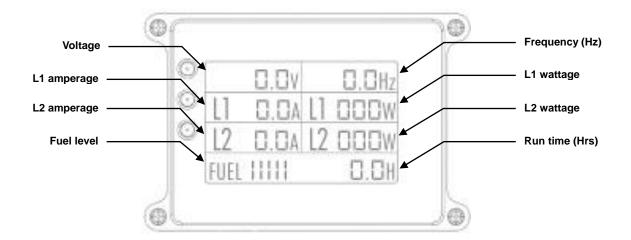
The digital display will illuminate within a few seconds of the generator starting, and will initially display data from the last run of the generator. Within a few seconds of illumination, the display will begin to show new data, and at that point the generator is ready to supply power.
