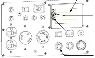
Digital display: The digital display illuminated and returning data indicates normal operating conditions.
