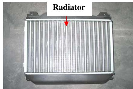
b. The engine cooling system is using closed cooling forced circulation system which mainly consists of radiator, sub water tank, water pump, heat-sensor switch, water holes, fan blade and fan motor.
