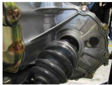
**Grade of gear box oil : SAE85W/95**
