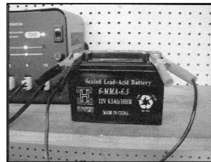
3.3) Charging rate: Charge battery @ 0.7 Amps for 5 ~ 10 hours;
