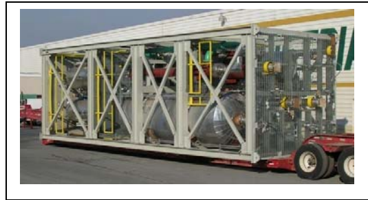
Dehydration Skid shop built and shipped to site.
