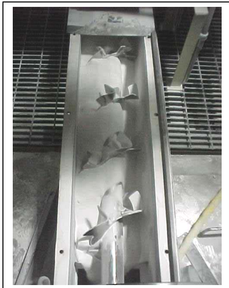
Mixing flights blend PVC virgin and regrind (screw trough cover removed)
