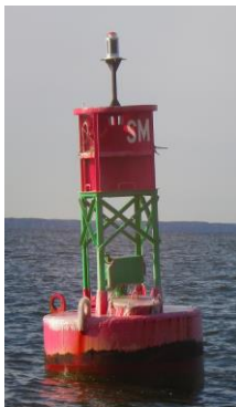
Red and white (safe-water) pillar buoy on station. Note the single spherical topmark.
