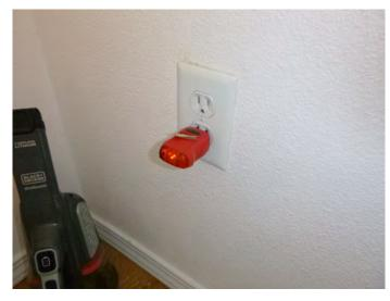
supply circuit are connected to the corresponding hot and neutral wires of the appliance. Contact a licensed electrical contractor for further evaluation and repairs.
