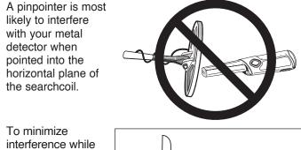
interference while probing the ground, lay the metal detector down with the searchcoil perpendicular to the ground.
