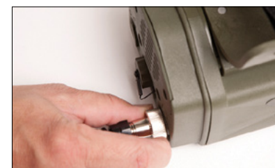
Hand-tighten connector collar.
