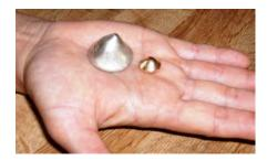
After the mold and the borosilicate glass have cooled, invert the mold and the conical shaped glass will drop out of the mold. The smelted metal "button" will be on top of the conical shaped glass. The glass splinters shooting from the "button" and glass can occur at any time until the metal "button" is completely free of the glass. So, keep everyone, pets included, out of the area. Hold the metal "button" in your gloved hand and tap the glass on the button with a
