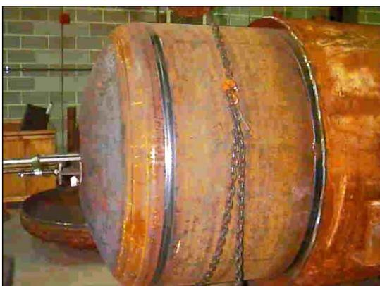
*The heart of your process is your Cooker. Proper alignment of the inner shell is critical for paddle clearance, keeping your inner shell clean. Alloy crews with decades of reshelling experience, use special alignment techniques to assure proper fit and alignment of your inner shell, maximizing cooking capacity of your cooker.*
