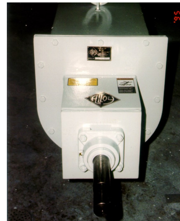
Alloy infeed screws incorporate an outboard flange block bearing, as seen here, to keep the materials being processed out of the bearing.
