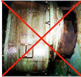
Most power pack drives in the industry have been mis-handled. To assure proper alignment, the cover needs to be line bored with the case that is to be used. In addition, the drive should be aligned and then pinned to maintain proper alignment. Most cookers have been rebuilt and serviced by persons not familiar with these requirements.
