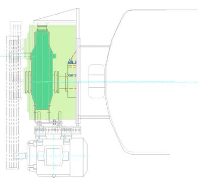
Alloy drive conversion package replaces the ANCO Power Pack drive with a Dodge shaft mounted, tapered bushing reducer, Dodge pillow block bearing, a bracket for the bearing and a bracket for the torque arm on the reducer. After conversion, wear parts are stock available from Alloy, Bearing houses or Dodge direct.
