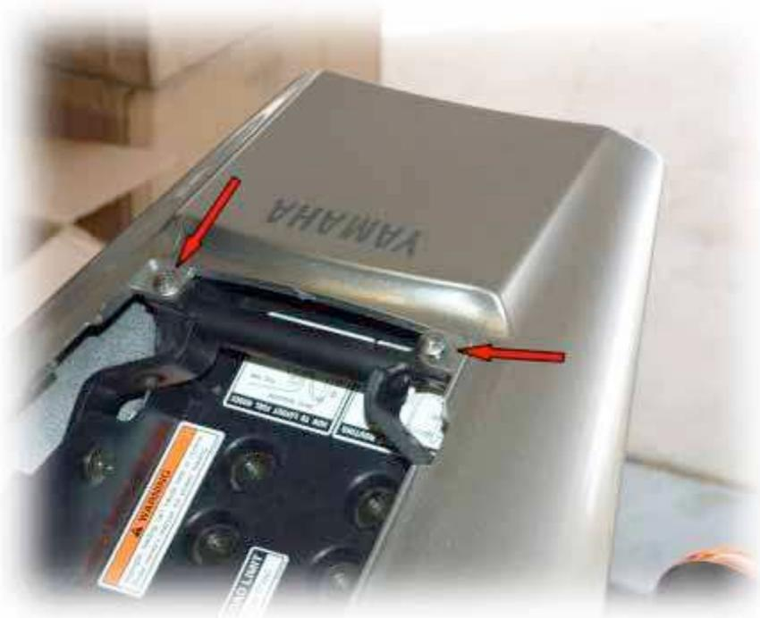
**3. Remove the tail section by removing the two upper metal screws under the rear seat and then remove the two plastic screws at the front of the tail section that are under the front seat. Next remove the six plastic snap rivets that are on the bottom of the tail section**
