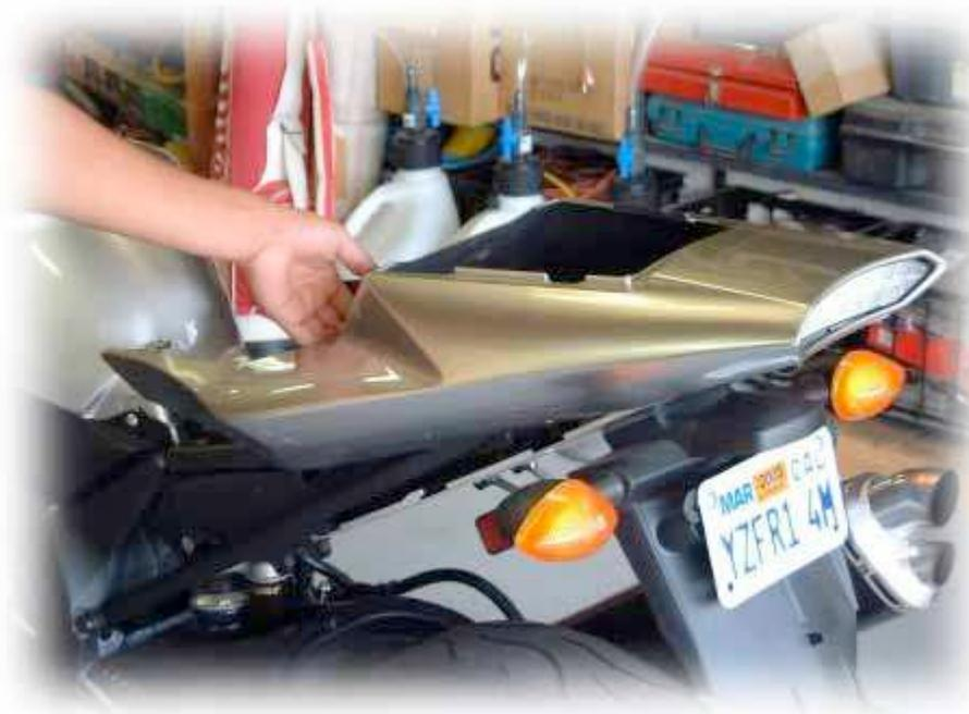
**4. Remove the stock undertail by first disconnecting the taillight group on the left hand side of the sub frame. Noting which connectors go to the left and right hand side turn signals, Grey (left hand signal) and Black (right hand signal) Then remove the four nuts from inside the storage compartment, making sure to support the tail lights. Remove the stock undertail and light group.**
