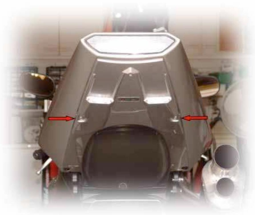
**9. If you plan to install the provided license plate bracket, slowly drill from to the outside the 4 holes meant to attach the bracket, use the OEM bolts and nuts, bolts outside and nut rack inside, upside down.**
