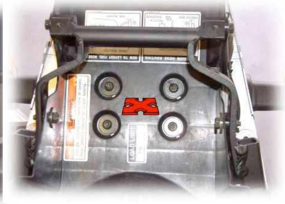
**5. The stock undertail will then have to be drilled to allow the new turn signal wiring to run into the stock wiring. Use a 5/16th drill bit and be sure to trim away any sharp edges after drilling.**
