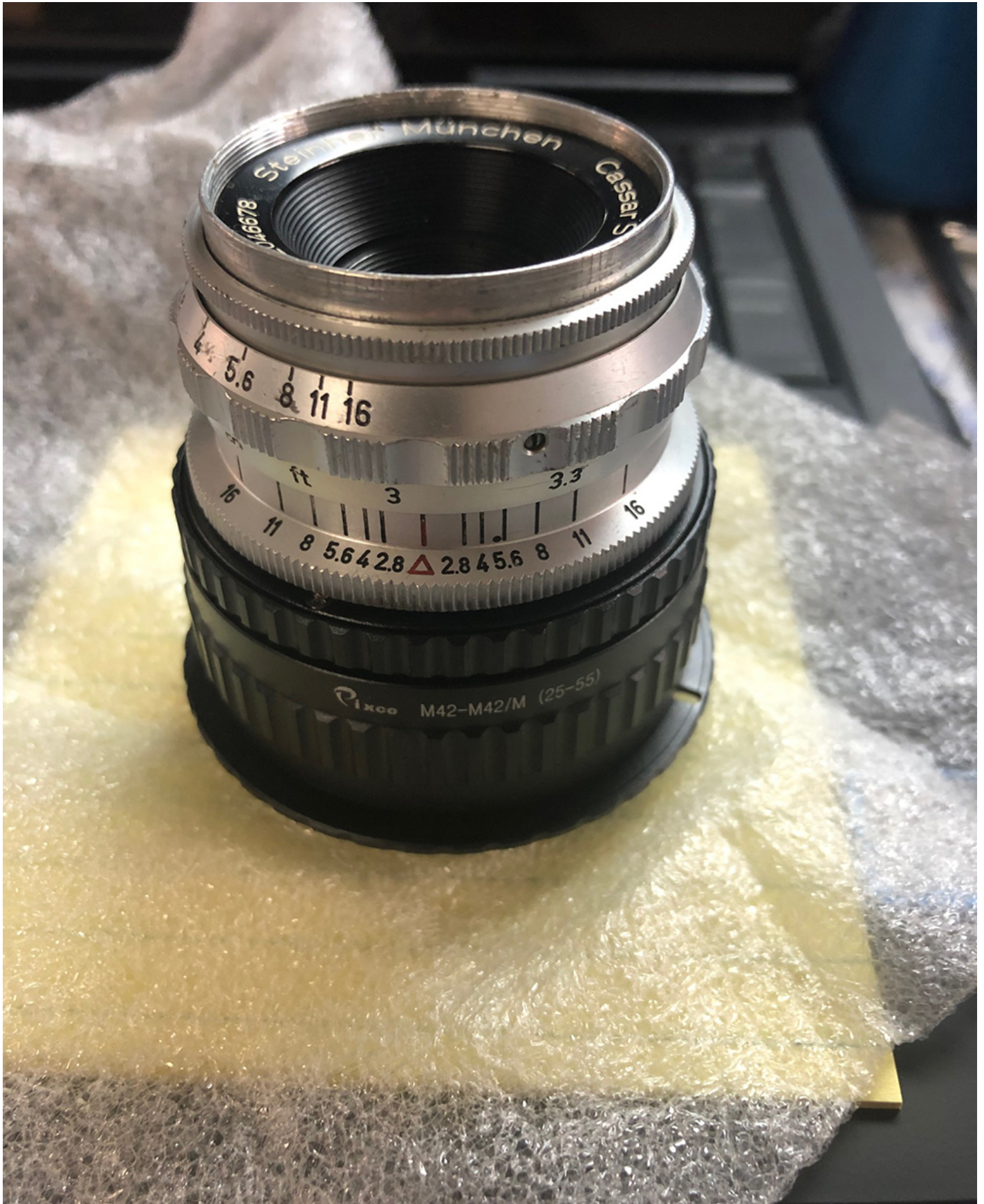
Figure 8 —Screw-mount lens with helicoid extension tube and DSLR camera mount. Image: Arthur H.
