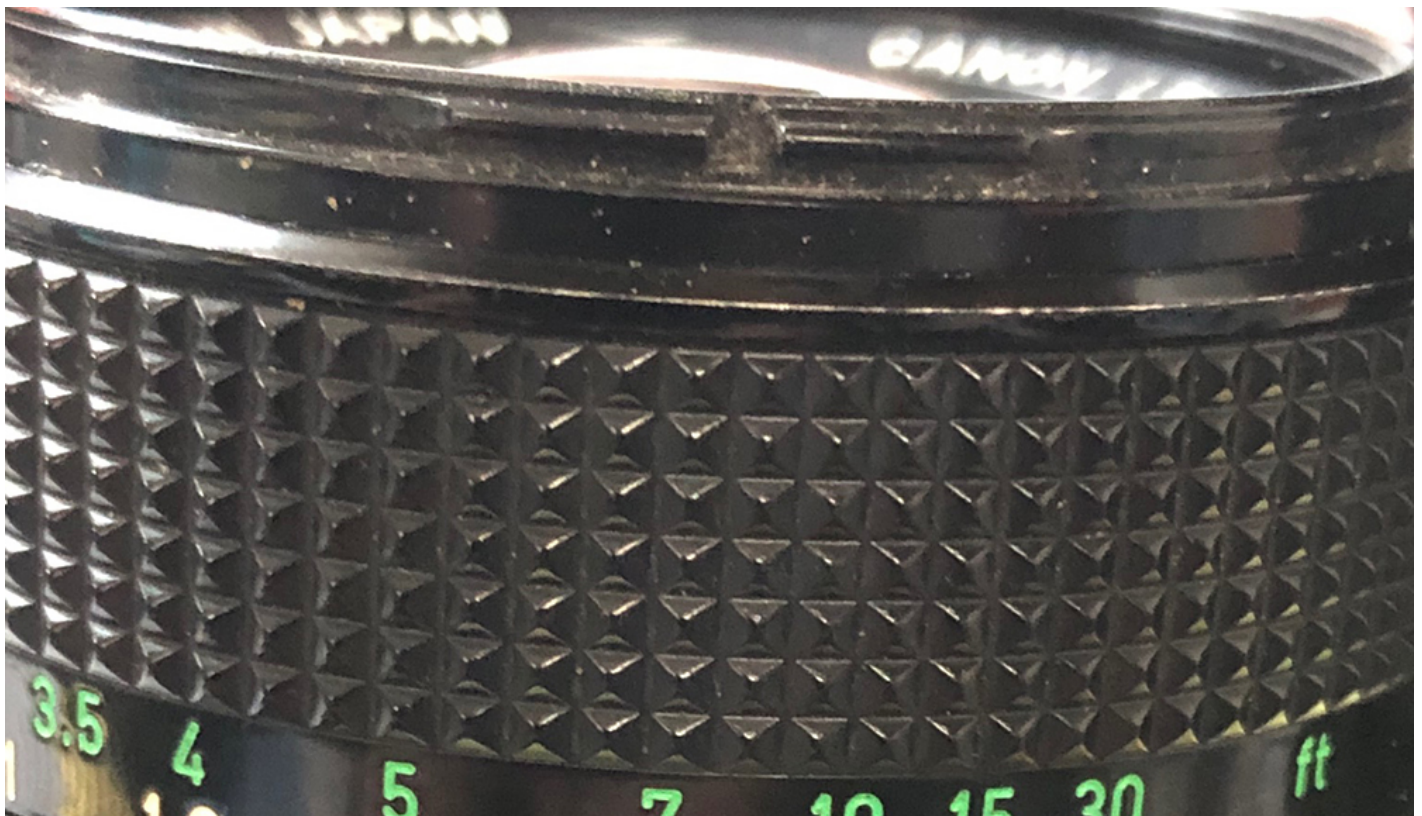
Figure 6 —Focus adjusted to align with IR dot. Image: Arthur H. Borchers
