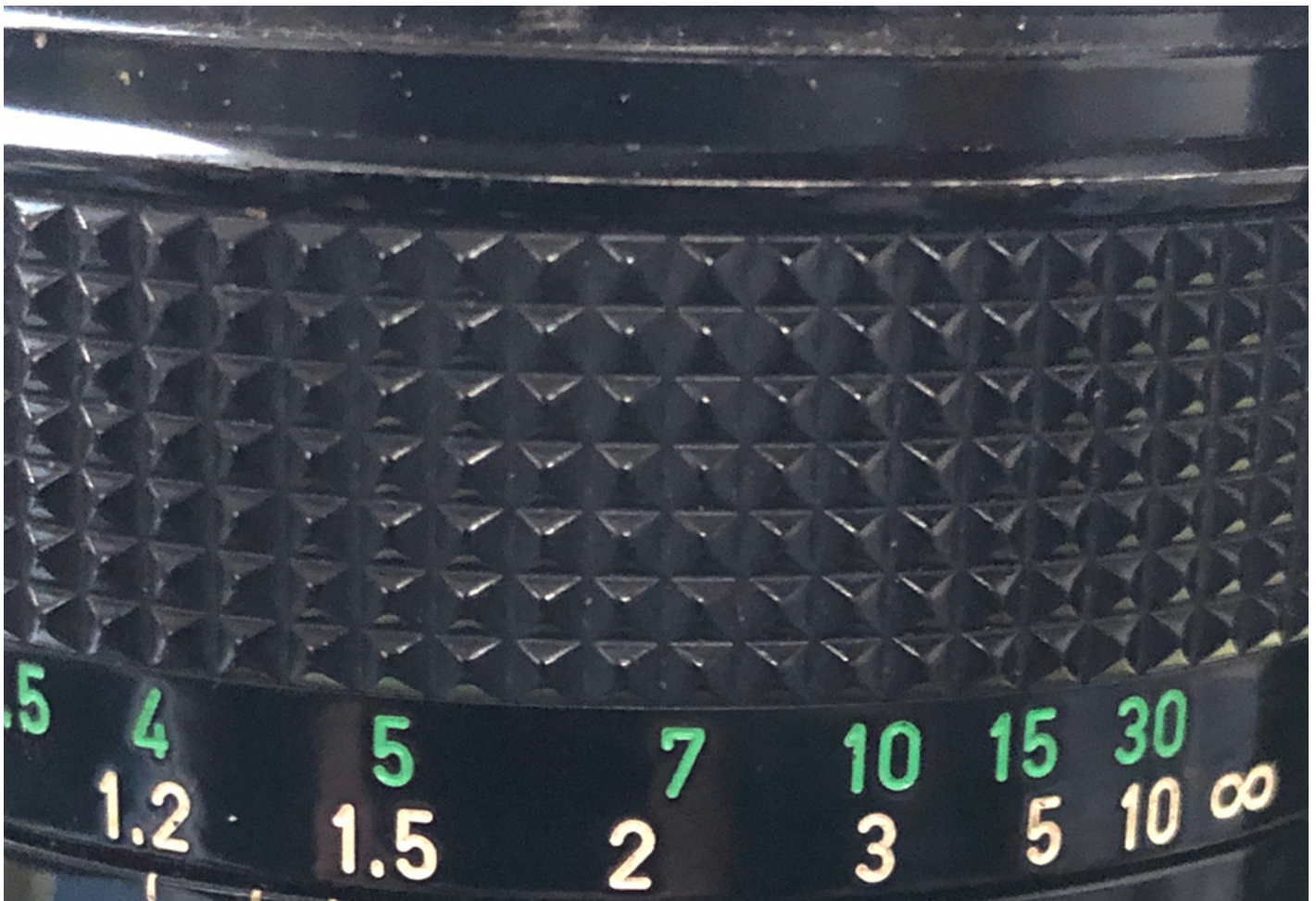
Figure 5 —IR focus dot to the right of f/4 depth of field mark. Image: Arthur H. Borchers
